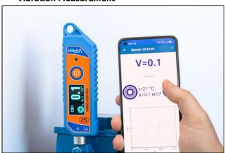
Vibration measurement with the ViPen device is carried out using a contact probe or a magnetic fastening block designed for use on flat and curved surfaces. The probe and the magnetic fastening block are fixed on the device body using a threaded hole.
