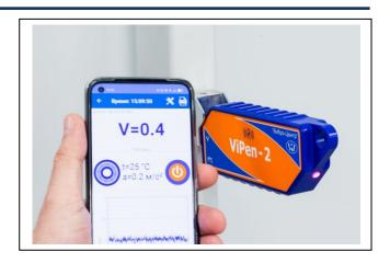
The device is controlled from a smartphone, for which special software is supplied together with the device.
